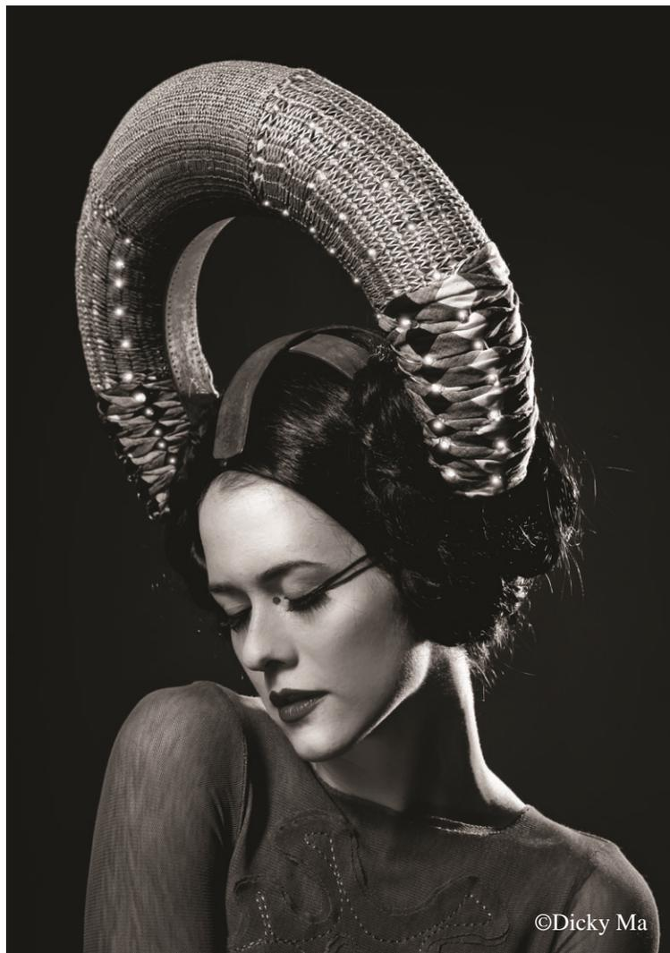
**Figure 1. Blinkifier, a wearable computer that amplifies human blinking**
